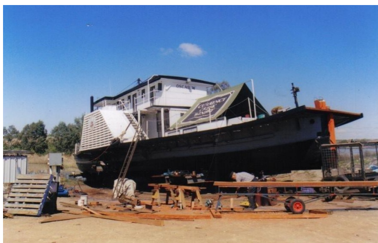
2004 Oscar W Slipped stern first at Mannum for restoration of stern timbers & frames
